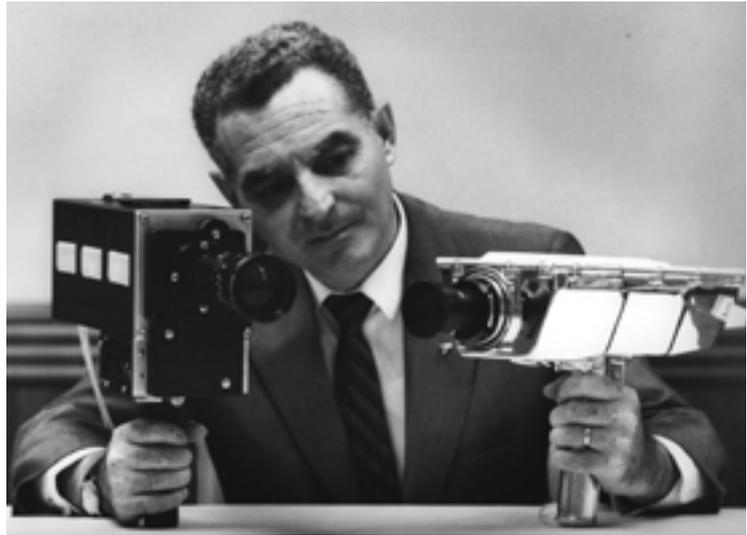
Stan Lebar, project manager for Westinghouse's Apollo television cameras, shows the field-sequential color camera on the left and the monochrome lunar surface camera on the right. NASA
